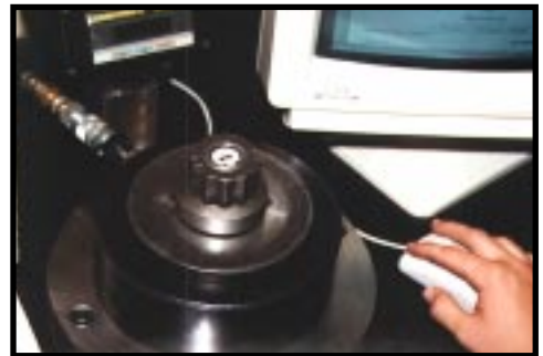
Every load indicating fastener is calibrated and tested to its proof load to assure accurate performance.
